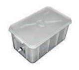
The condensate neutralisation system is an accessory for the condensing boilers. The acid condensate must be neutralised with calcium carbonate to bringing the pH values above 7 thus allowing the discharge together with the domestic water according to the prevailing laws. It is available in two versions with container and 25 kg of calcium carbonate beads.
