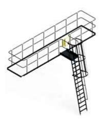
The structure consists of carbon steel profiles connected by special joints that ensure their correct coupling.
